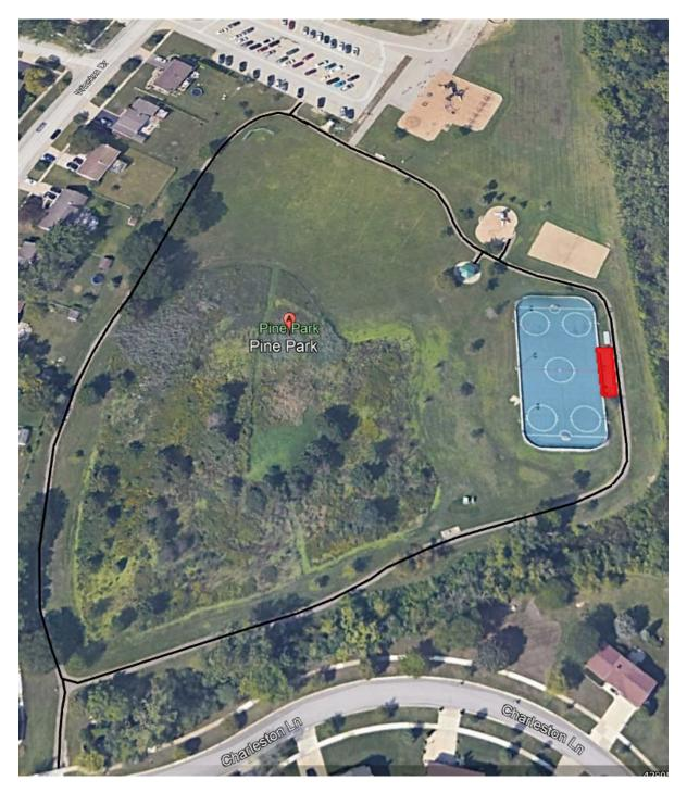
Existing path is 2100 linear feet by 8 feet wide (black lines). The red highlighted area is an existing asphalt pad that is part of the path that is 60 linear feet by 15 feet wide. There is a total of approximately 17,700 square feet of paving to milled and overlaid. For exact measurements it is recommended to visit the site prior to bidding on the project.
