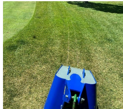
After running the root pruner the only evidence is two faint lines.
