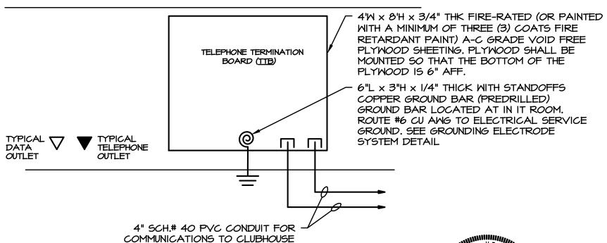
DETAIL - TELEPHONE/CATV RISER 'TTB' NOT TO SCALE
