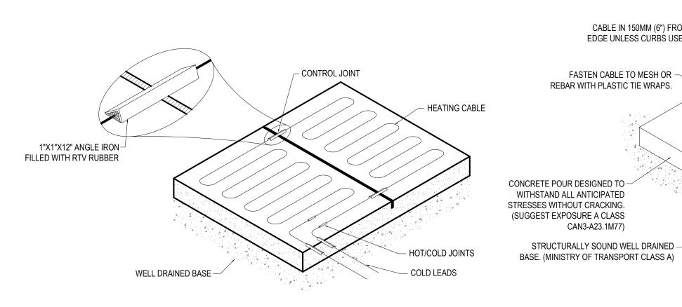
METHOD OF CROSSING CONTROL JOINT WITH M.I. HEATING CABLE IN CONCRETE SLAB
