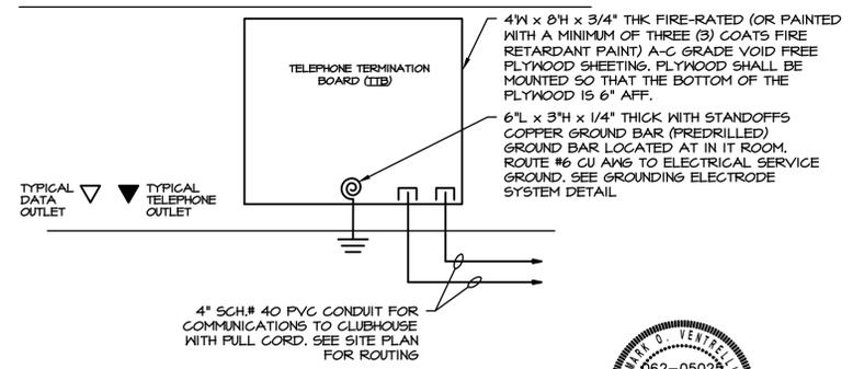
**DETAIL - TELEPHONE/CATV RISER 'TTB'**
